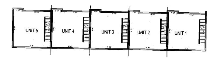
FLOOR PLAN - GROUND LEVEL Elevations on this level are between 504,4583' and 514,4583' based upon a finished floor elevation of 504,4583' at ground level.
