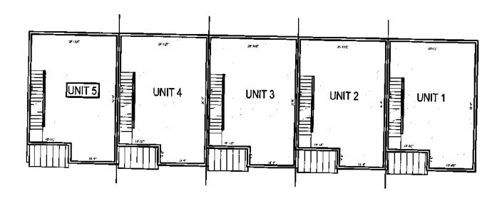
FLOOR PLAN - SECOND LEVEL Elevations on this level are between 509,8749' and 524,5416' based upon a fluished floor elevation of 504,2083' at ground level
